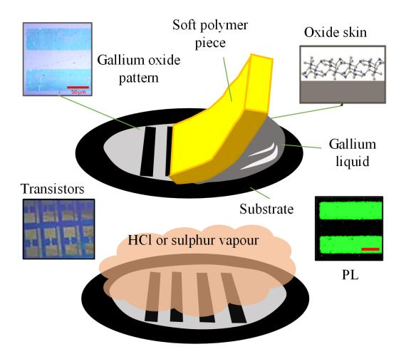
Figure 1: The demonstration of the fabrication process of 2D gallium oxide from gallium liquid metal and transformation of this material to lower bandgap semiconducting 2D gallium sulphide
