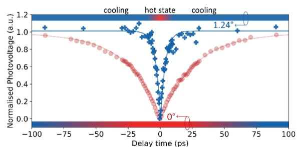
**Figure 2:** Controlling the time delay between two ultrafast pulses reveals the hot carrier cooling dynamics. At low temperatures, these are significantly faster in the case of MATBG ( $1.24^\circ$ ) than non-twisted BLG ( $0^\circ$ ).
