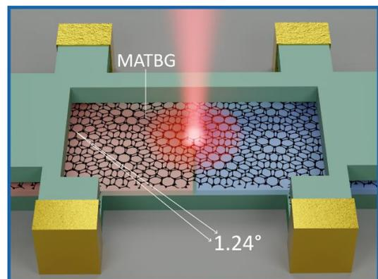
**Figure 1:** Illustration of the hBN-encapsulated MATBG device with twist angle  $1.24^\circ$ . We generate a photovoltage by illuminating the electrically defined pn-junction ( $\pm V$ , red/blue regions).
