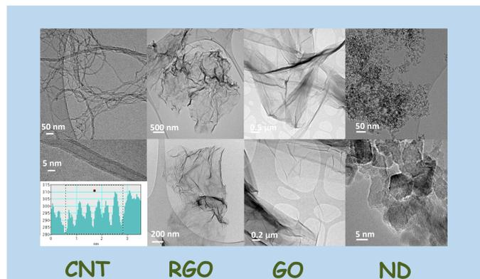
Figure 1. Transmission electron microscopy (TEM) characterization of the carbon nanomaterials tested here. The CNT used here are relatively short MWCNT (up to 1 micron in length) and ~10 nm in diameter, comprising around six concentric nanotubes. TEM micrographs of two-dimensional, graphene derivatives GO and RGO reveal that most flakes are up to 1 micron in length as well as their high exfoliation degree. Finally, Figure 1 shows aggregates comprising ND of about 5 nm in diameter.
