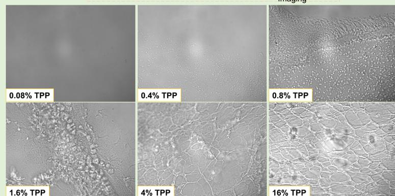
Figure 6. TPP promotes the formation of porous hydrogel-like PAEtMA-CI in water.
