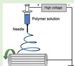
Figure 3. Schematic illustration of electrospinning apparatus used to produce poly(AEtMA) fibers.
