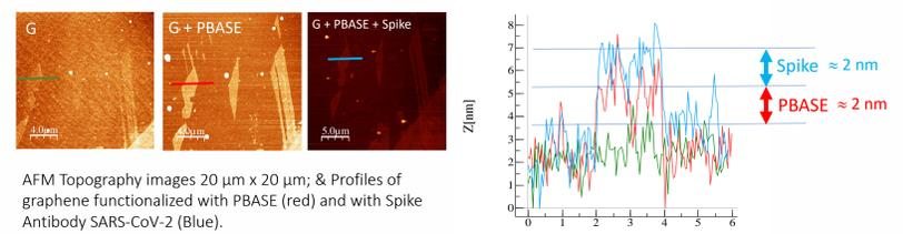
AFM Topography images 20 μm x 20 μm; & Profiles of graphene functionalized with PBASE (red) and with Spike Antibody SARS-CoV-2 (Blue).
