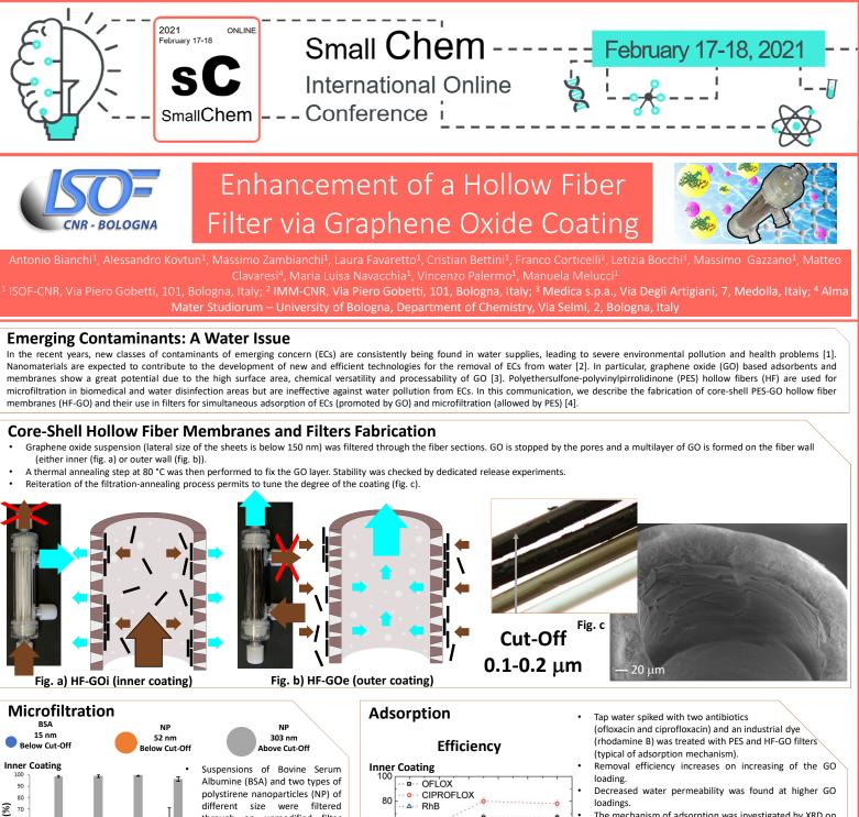
The mechanism of adsorption was investigated by XRD on the fibers before and after filtration and by theoretical calculations. Experimental and theoretical data suggest intercalation of ofloxacin in between overlapped GO sheets
