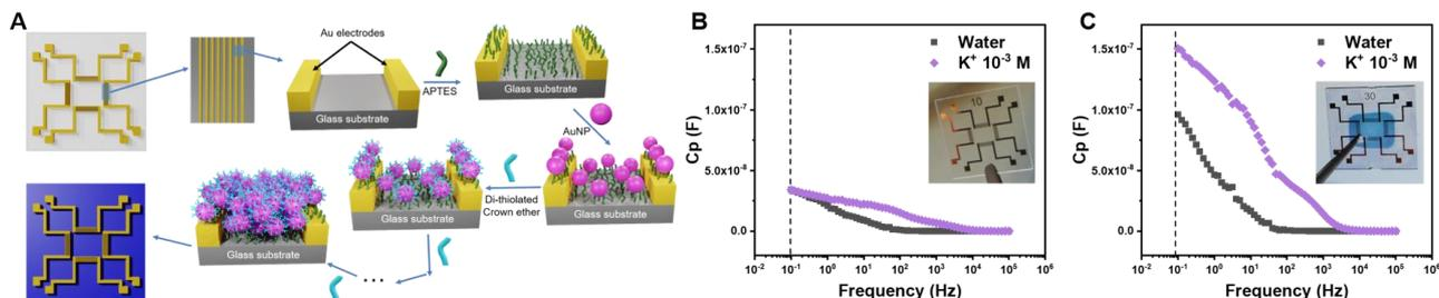
**Figure 1:** (A) Schematic representation of AuNP-dithiolated crown ethers assemblies fabricated by Layer-by-Layer deposition, (B-C) Capacitance response of devices in water (black curves) or  $K^+$   $10^{-3}$  M (purple curves) in the absence (B) or presence (C) of the 3D network of AuNPs. The inset show the optical image of the device without (B) and with (C) the 3D network of AuNPs.
