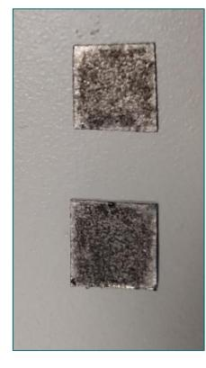
The obtained CNTs where dispersed inside the ethanol electrolyte that contains the NiO nanoparticles to be sprayed later on top of graphite substrate to use it as electrode for supercapacitors.
