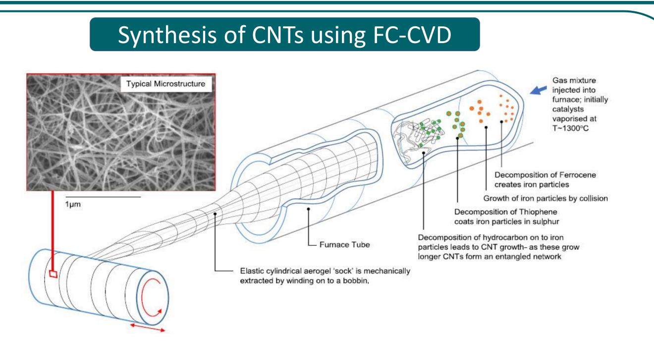
The setup used to obtain continuous CNTs mats which explains the steps starting from the injection of ferrocene, methane, and thiophene at a temperature above 1200C. [3]
