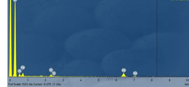
Characterization of the morphology of the CNTs using: (a,b) SEM which shows the thickness of the CNTs mat which ranges between 1.40 um and 2 um. (c) EDS for microstructural analysis which shows short peaks of iron (Fe) which comes from the ferrocene and sulfur which produced from the decomposition of thiophene.
