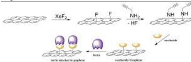
**Figure 1:** Functionalization of graphene, covalent grafting of carbohydrates and selective binding of WGA.
