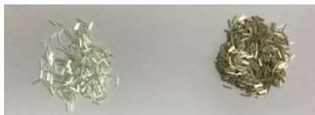
Figure 1: Uncoated and rGO-coated glass-fibers for polymer composite reinforcement.
