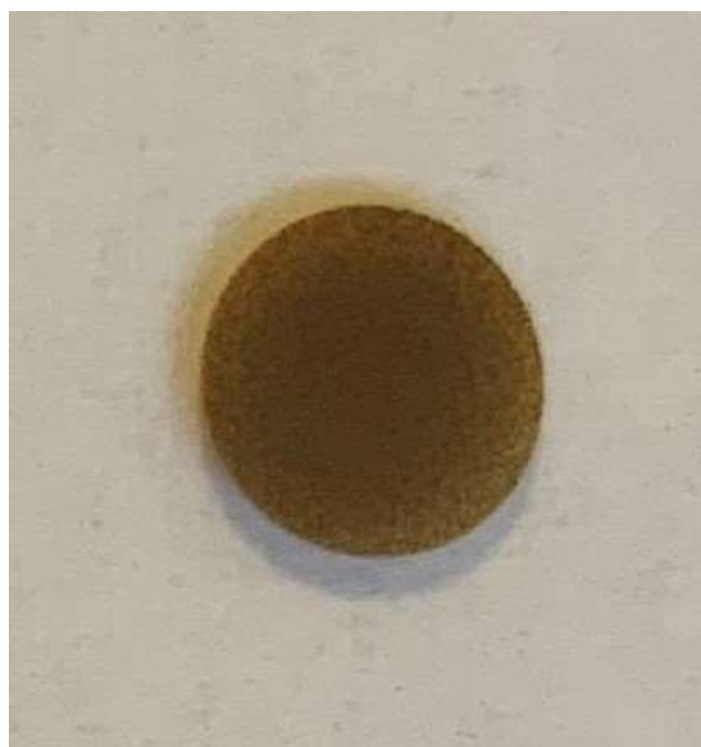
Figure 2: rGO-coatings on borosilicate glass-slide prepared by electrospaying.
