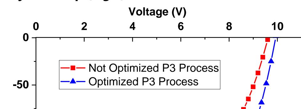
The Graph shows how P3 process impacts on module performance. The **red I-V curve** is acquired on a module with **not optimized P3** process. The incomplete gold removal reduces the module maximum voltage and FF. By performing a second **optimized P3** process on the same module, the efficiency was boosted up to **15,3%** (blue curve)
