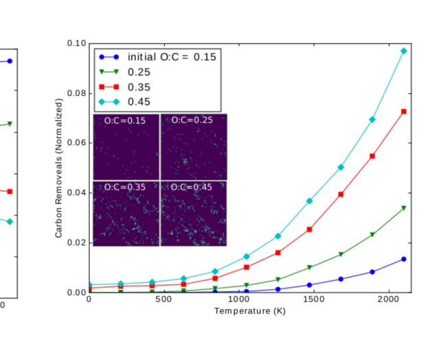
The increasing number of vacancy formations could even engender the removal of the entire oxidized area leaving a hole
