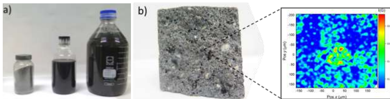
Figure 1: a) Examples of graphene dispersions produced by the wet-jet milling process. b) Raman mapping image of the fracture surface of a few layer graphene-based cement mortar sample.
