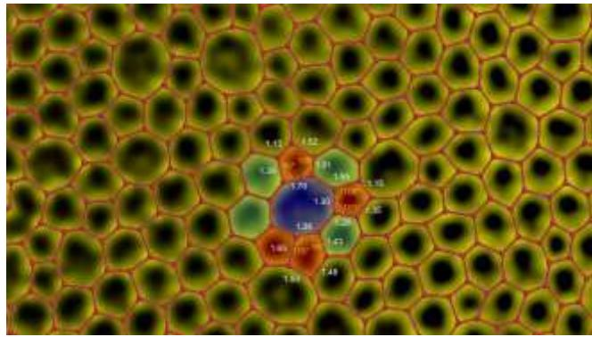
**Figure 1: Atomic structure of MAC from TEM.** Monochromated HRTEM image of MAC. The image contrast is inverted and false-coloured for better visibility. Colour overlay is added for identification of pentagons (red), heptagons/octagons (blue) and strained hexagons (purple for individual hexagons; green for crystallite regions) that are omnipresent. Crystallites (regions of green hexagons) separate the regions with non-hexagons.
