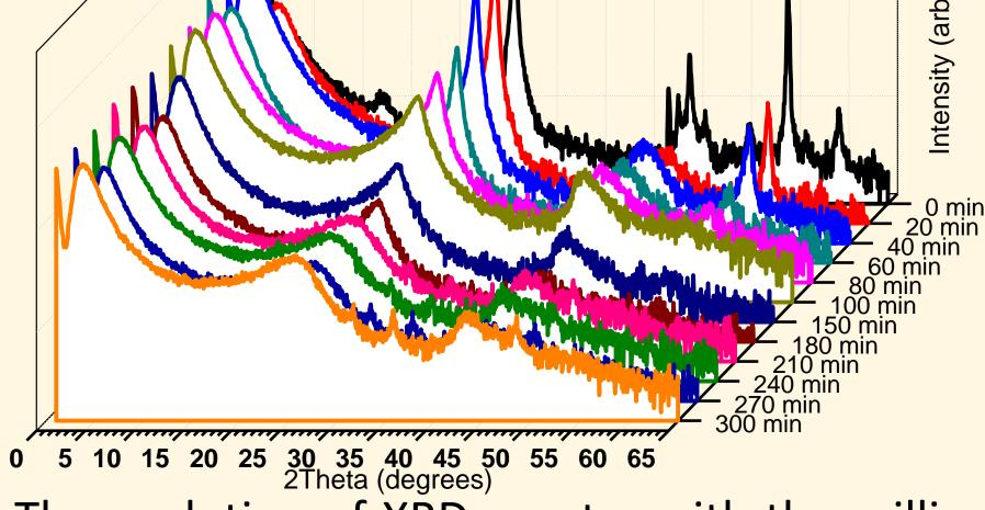
The evolution of XRD spectra with the milling time show the decrease of 26.5° [002] maximum, associated with the exfoliation process of graphite.
