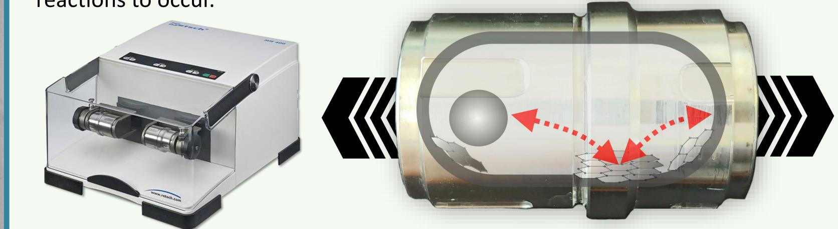
We used graphite as a precursor with no added elements (neither liquid medium nor additives), thus requiring no additional treatments. Graphite suffers exfoliation and defects formation during the process.
