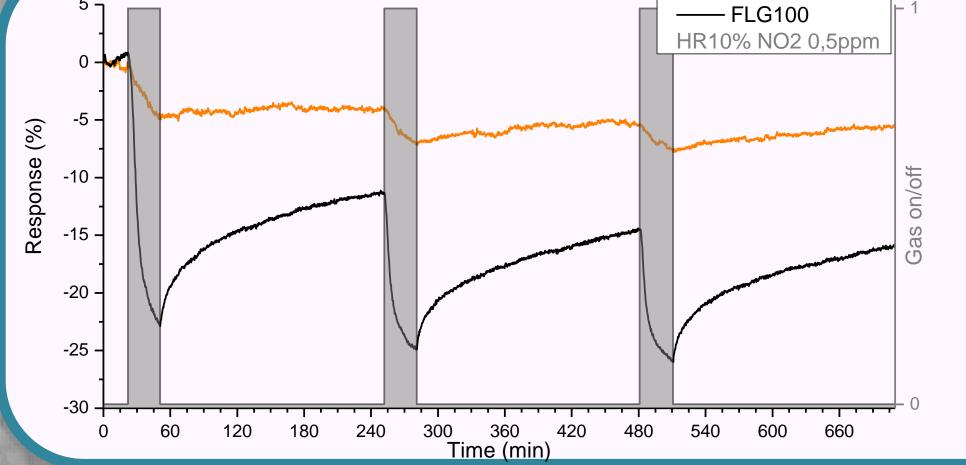
Furthermore, the obtained FLMG is reproducible and valuable. High specific surfaces and defects on graphene-based materials are desired for various applications such as gas sensing, where FLMG demonstrated excellent performance compared to standard graphite [3].
