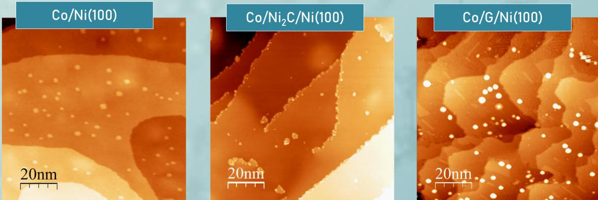
**Cobalt on Ni(100):** Co grows in randomly distributed 2D-islands following the 4-fold symmetry of the (100) substrate. Stability increases with increasing number of atoms.
