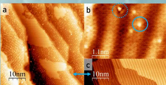
Co doped graphene, a: Graphene grown during Co evaporation, b: atomic resolution suggesting two different dopant configurations, c: Graphene on Ni(100) without Co evaporation.
