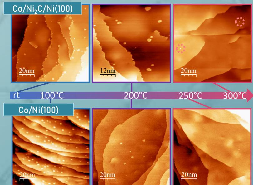
STM measurements at elevated temperatures (up to 500°C) allowed us to investigate Co stability on the surface. In case of Ni<sub>2</sub>C, Co remains on the surface up to 300°C (marked in pink circles) for more than 1 h. Whereas on bare Ni, alloy formation starts at 150°C and Co islands vanish after 1 h at 250°C. Numerical simulations confirmed these observations, predicting a lower barrier for Co penetrating the Ni surface than Ni<sub>2</sub>C.
