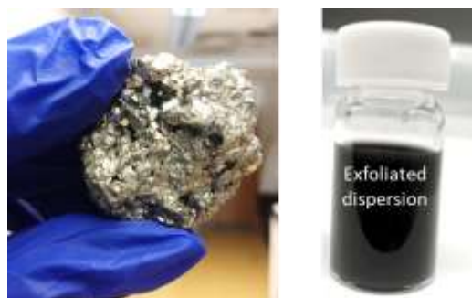
Figure 2: Liquid phase exfoliation of the mineral, fool's gold (pyrite).
