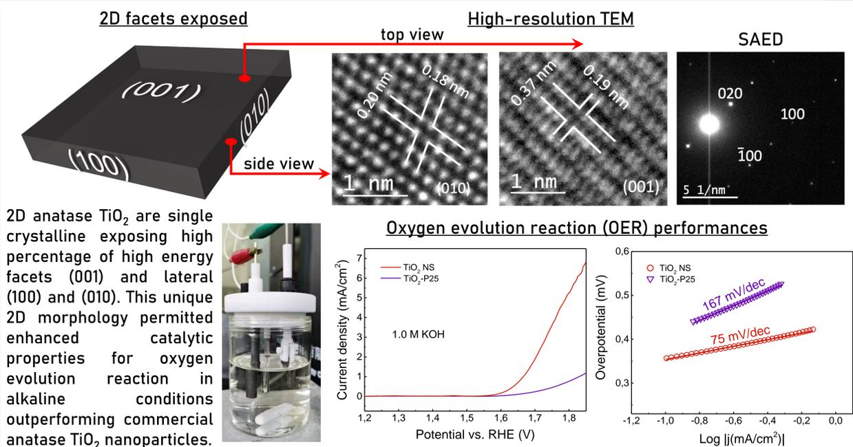
2D anatase TiO<sub>2</sub> are single crystalline exposing high percentage of high energy facets (001) and lateral (100) and (010). This unique 2D morphology permitted enhanced catalytic properties for oxygen evolution reaction in alkaline conditions outperforming commercial anatase TiO<sub>2</sub> nanoparticles.
