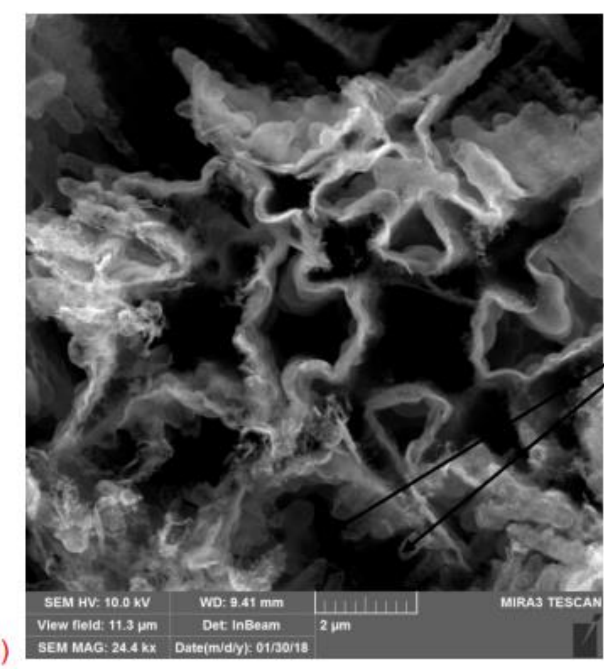
SEM images of porous silicon samples. Arrows indicate the Graphene layers on the surface of pores of skeleton PS
