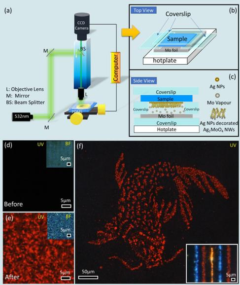
Laser assisted selective seeding of Ag NPs on GO film for the growth of hybrid  $\text{Ag}/\text{Ag}_2\text{MoO}_4$  NWs on hotplate.
