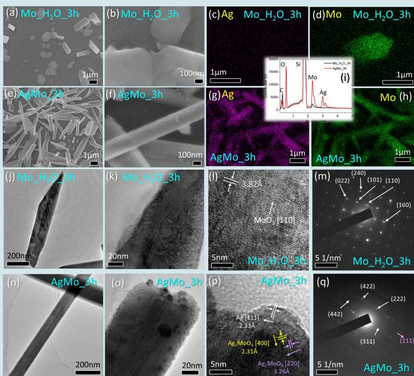
**Figure 2.** (a,b,e,f) SEM of (a,b)  $\text{MoO}_3$  nanobelts and (e,f)  $\text{Ag}/\text{Ag}_2\text{MoO}_4$  NWs. (c,d,g,h) EDX elemental map of (c,g) Ag and (d,h) Mo from (c,d)  $\text{MoO}_3$  nanobelts and (g,h)  $\text{Ag}/\text{Ag}_2\text{MoO}_4$  NWs. Inset is the corresponding spectrum obtained from both samples. TEM, HRTEM and SAED images of (j-m)  $\text{MoO}_3$  nanobelts and (n-q)  $\text{Ag}/\text{Ag}_2\text{MoO}_4$  nanowires.
