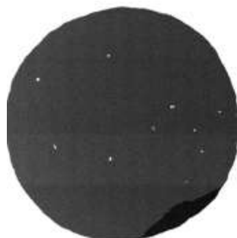
Free standing graphene on grid hole (Diameter 1.2 μm)
