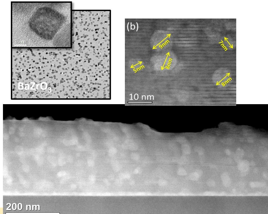
Integrating nanocomposite in coated conductors with cost effective processes for power applications and magnets
