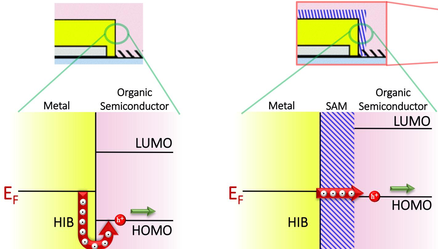
Charge injection barrier in OFETs can be overcome by tuning **work function** of metals, by the presence of an interfacial dipole created by organic molecules arranged on the metal surface as **Self Assembled Monolayers (SAMs)**.
