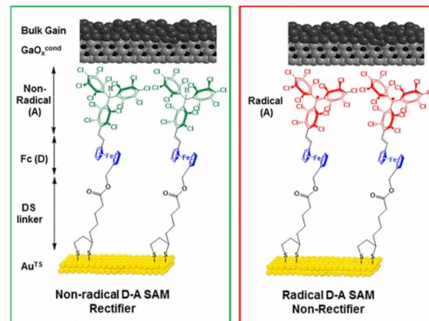
Influence of the donor unit on the rectification ratio in tunnel junctions based on donor–acceptor SAMs using PTM units as acceptors
