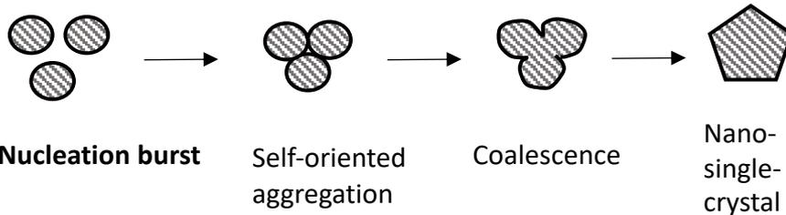
➤ Fine control of the nanocrystallisation process
