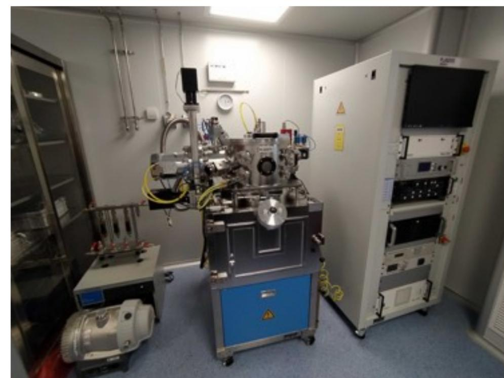
Ebeam deposition system for qubit production
