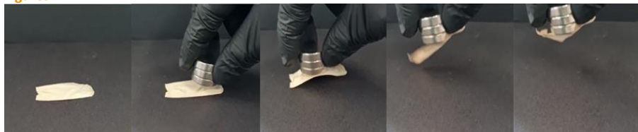
Figure 1: Sequence of digital images of the magnetic response of an electrospun membrane with \text{Fe}_3\text{O}_4 nanoparticles.
