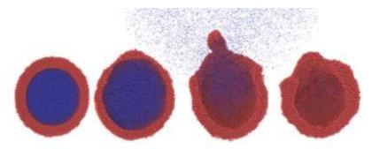
Molecular dynamics simulations of a hollow tungsten nanosphere explosion highly pressurized at 3000 K. Red = W atoms, Blue = Helium atoms.
