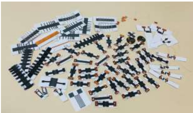
Figure 1: Picture of several paper-electronic devices fabricated by integrating different van der Waals semiconductors on standard copy paper substrates.
