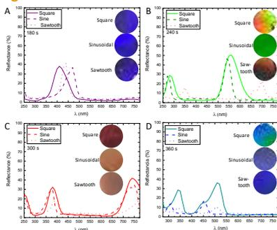
**Figure 1:** UV-Vis reflectance spectra as a function of the wavelength of 3D-AAO nanostructures or different waves and rest times. (a) 180 s, (b) 240 s, (c) 300 s, and (d) 360 s. In the inset, optical images of 3D-AAO colour for different waves and resting times were studied.
