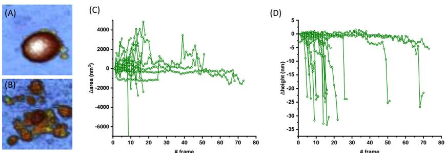
**Figure 1:** Evolution of an individual CP particle under mechanical fatigue procedure. (A) Frame #0 shows the intact particle, (B) frame #12 is the image of the final collapsed state. (C) Evolution of the particle surrounding covered area with debris for CP VLP. (D) Evolution of the particle height for CP virus particle.
