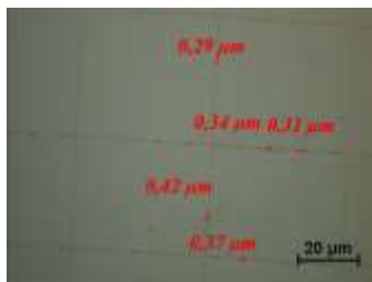
Figure 1: Deposition pattern of fibers formed by near-field electrospinning method
