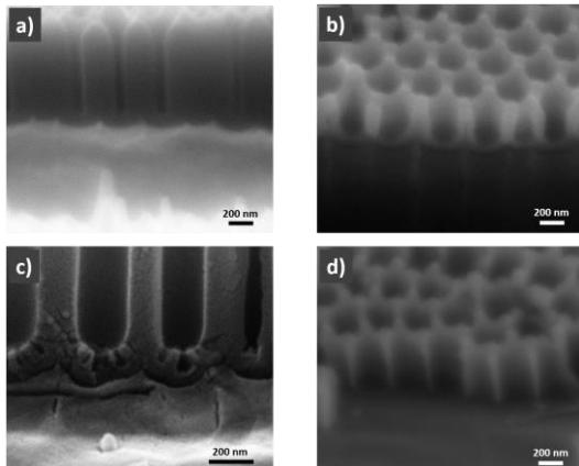
**Figure 1:** Cross-section views SEM of a phosphoric NAA **a)** after the two step anodization. **b)** after the partial pore widening. **c)** after re-anodization at constant current. **d)** after final pore widening. Sacles are indicated in the pictures.
