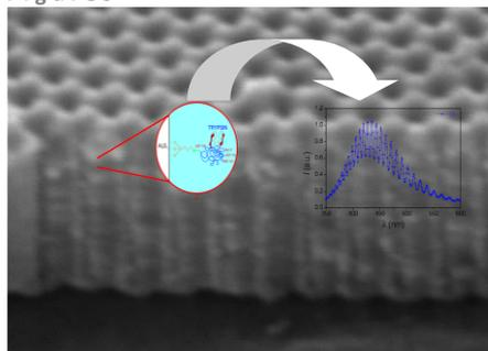
**Figure 1:** Cross-section SEM image of NAA. Inset: schematic illustration of the chemical functionalization of the pore surface and reflectometric interference spectroscopy spectrum of NAA. Pore diameter = 45 nm.
