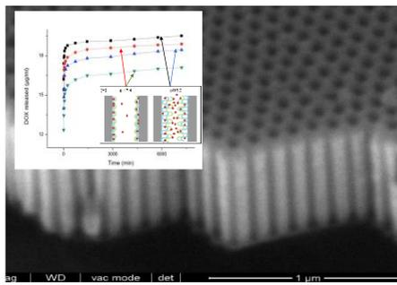
**Figure 2:** SEM image of NAA. Inset: DOX release at pH 5.2 and 7.4 for NAA (black and red symbols) and NAA coated with a PH stimuli-response polyelectrolyte (blue and green symbols).
