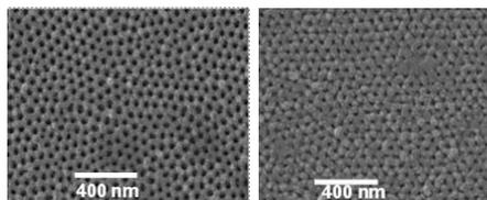
Figure 1: SEM top view images of: NPAMs (left); NPAM+SiO<sub>2</sub> (or NPS) (right).
