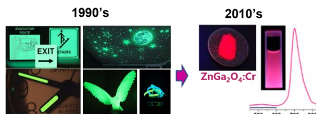
Figure 1. Green PERL bulk materials in the 1990's vs Near Infrared PERL nanoparticles in the 2010's.
