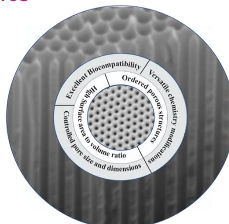
**Figure 1.** SEM image of an NAA cross-section and major features.
