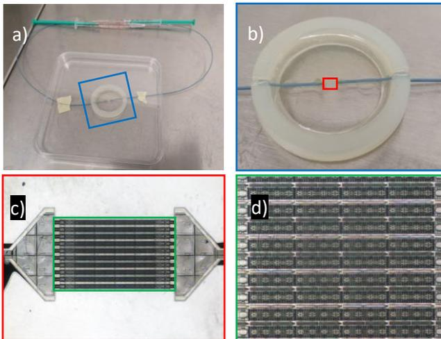
**Figure 1.** 3D microfluidic BBB system. a,b) System connected to syringes. c,d) Microscope images of the porous microtubes in parallel. Endothelial cells can be seeded inside or outside the microtubes to mimic blood microcapillaries.
