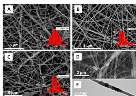
**Figure 2:** SEM micrographs of electrospun mats. A) PCL, B) PCL-CS, C) PCL-CS-TiO<sub>2</sub>TX. Insets show the corresponding fiber diameter distribution. (D) SEM Imagen of PCL-CS-TiO<sub>2</sub>TX mat without being coated in gold. (E) Imagen TEM of a single fiber of PCL-CS-TiO<sub>2</sub>TX.
