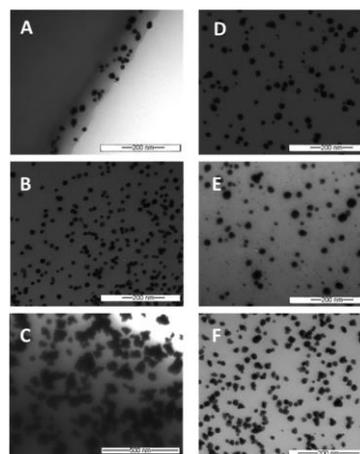
**Figure 1:** A- TEM images of gold-chitosan nanocomposite films obtained from immersion into different KAuCl<sub>4</sub> solutions. (a, d) 5%, (b, e) 10%, and (c, f) 20% of KAuCl<sub>4</sub> and reduced with hydrazine (left side) and L-ascorbic acid (right side).
