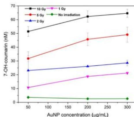
**Figure 2:** The effect of different AuNPs concentrations on the generation of 7-OH-coumarin (mean value ± SD of triplicate measurements) at different radiation doses. The solid lines connecting the data points are for guiding the eye.
