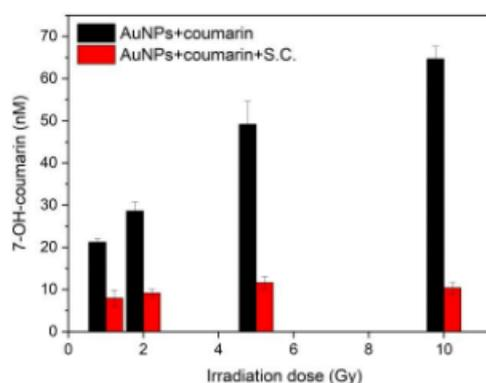
**Figure 4:** Amount of 7-OH-coumarin formed in the presence and absence of sodium citrate (S.C.) showing that the enhancement effect is due to the radical production which is significantly quenched in presence of the citrate molecules (AuNP+Coumarin+S.C.) (mean value ± SD of triplicate measurements).
