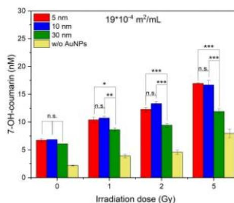
**Figure 3:** Amount of 7-OH-coumarin formed during the proton irradiation of water phantoms with different sized AuNPs at a constant total surface area of  $19 \cdot 10^{-4} \text{ m}^2/\text{mL}$  at irradiation doses of 0, 1, 2, and 5 Gy for the evaluation of the size/mass effect (mean value ± SD of triplicate measurements).
