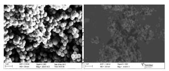
The contents of PCM vary in the 55 - 76 % range and the size of the microcapsules obtained are around 50  $\mu$ m. Magnetic measurements of the PCMs with embedded MNPs leads to the estimation of the amount of NPs loaded in the PCMs.
