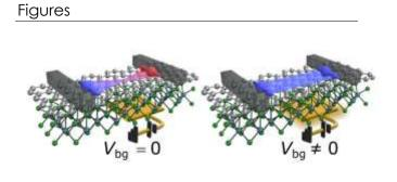
**Figure 1:** Sketch of a spin field-effect transistor operating at the strong spin-orbit coupling regime, where the valley-Zeeman induced spin precession is tuned by a back gate voltage to control the sign reversal.
