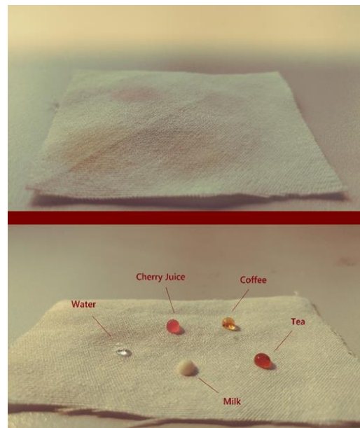
Figure 2: The behavior of the liquids with different properties on the standard and waterproof surface
