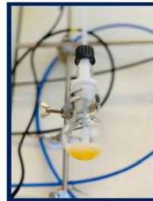
Figure 2: Lab-scale reactor for the production of graphene-doped Epoxy resin concentrates (Masterbatch)
