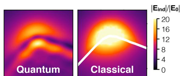
**Figure 1:** Zoom-in of the near-field maps around the tip of a Na icosahedral nanoparticle illuminated with linearly polarized light, at the energy of the dipolar plasmon, as calculated using TDDFT (left) and BEM (right).
