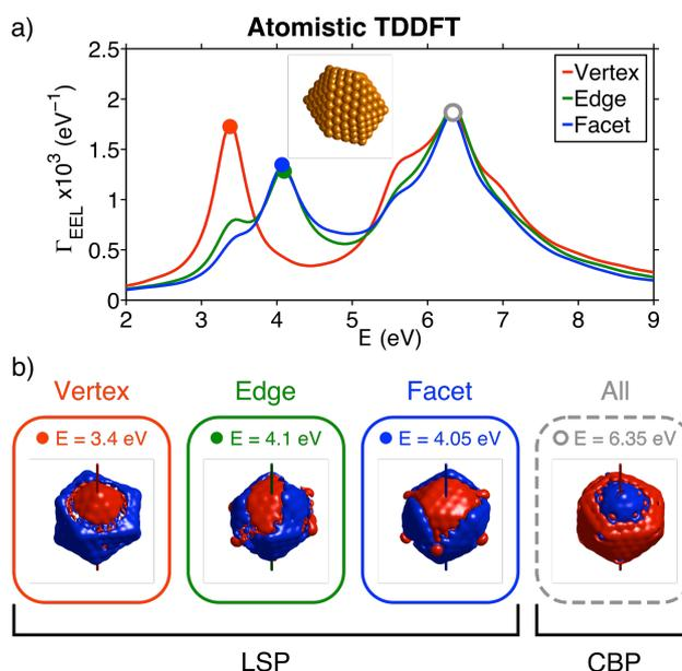
**Figure 2:** Electron energy loss spectra for the Na icosahedral cluster calculated using TDDFT for electron trajectories penetrating the NP through different atomic-scale features. b) Charge density isosurfaces corresponding to the main excited plasmon modes for each trajectory.
