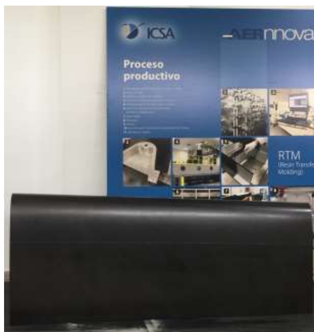
Figure 1: Horizontal Tail Plane Leading Edge prototype containing GRM manufactured by RTM
