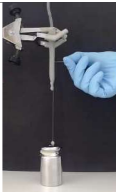
Figure 1: Hydrogel-based Mackibben muscle with self-healing properties.
