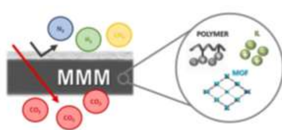
Figure 1: SEM image and schematic representation of a three-component mixed matrix membrane consisting of poly(ionic liquid) (PIL), ionic liquid (IL) and porous filler (MOF).
