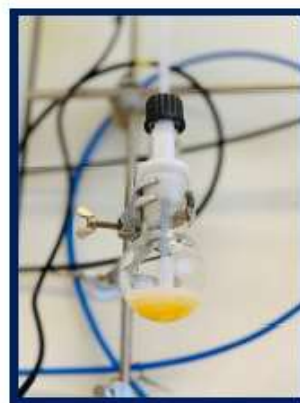
Figure 2: Lab-scale reactor for the production of graphene-doped Epoxy resin concentrates (Masterbatch)
