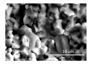
**Figure 2:** Micrograph of the Ti (C, N)-nNi structrure after presureless sintering.
