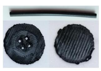
**Figure 1:** Filament and green pieces of Ti (C, N) with diferent shapes.
