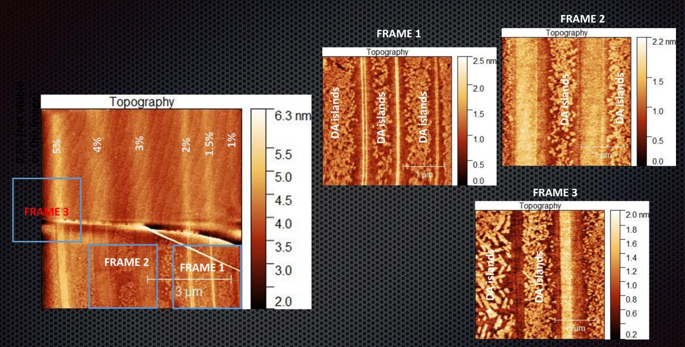
Typical patches of molecules seen only away from the irradiated lines! Molecules are repelled from all irradiated areas regardless of He dose! Need to compensate for the accumulated charge in the substrate
