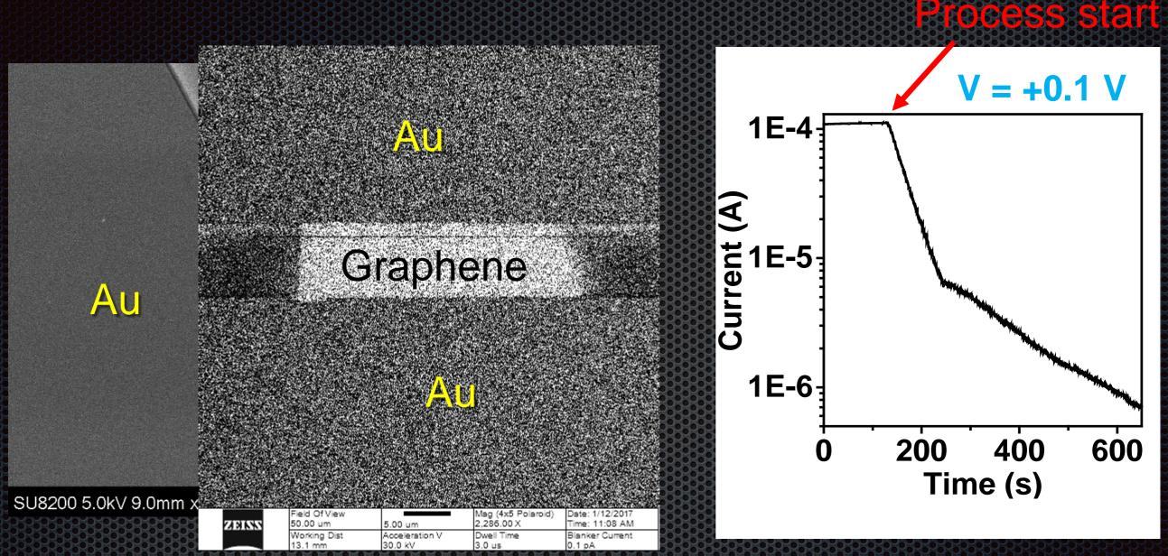
Irradiated a 100 nm-wide band, in 1 nm steps, across the full graphene flake.
