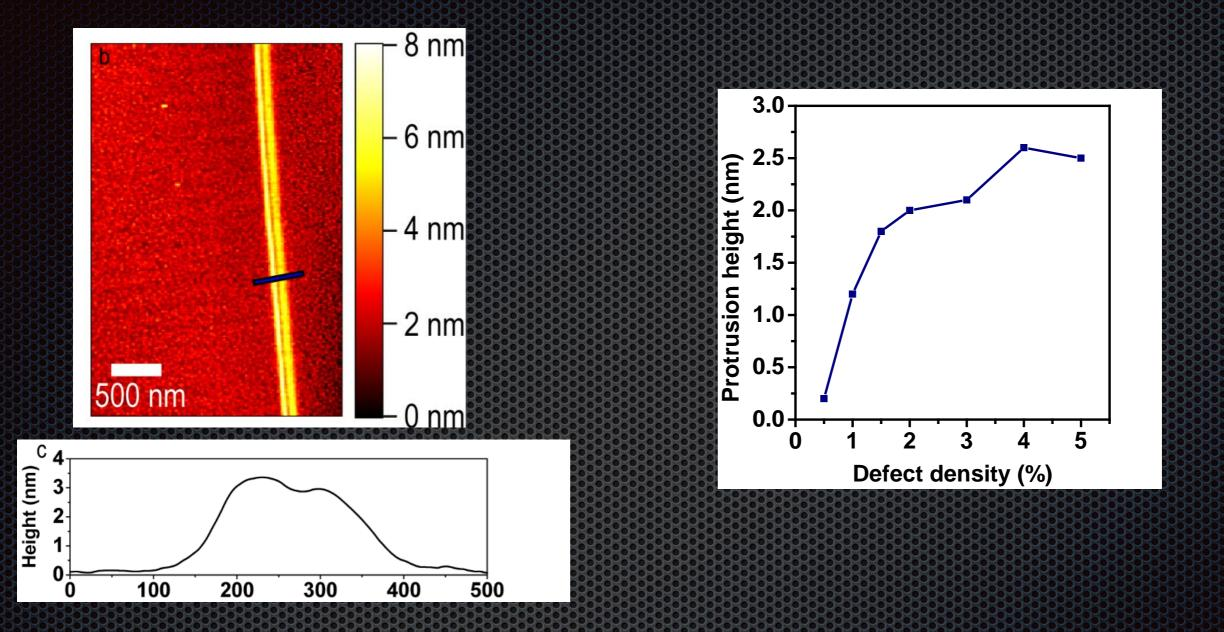
AFM indicates differences of designed vs. irradiated band size
